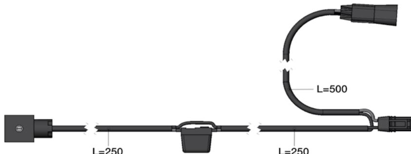
KIT CABLAGGIO CON CONNETTORE A TENUTA STAGNA, SENSORE DI TEMPERATURA MPC E VARIATORE ELETTRONICO DI VELOCITÀ
